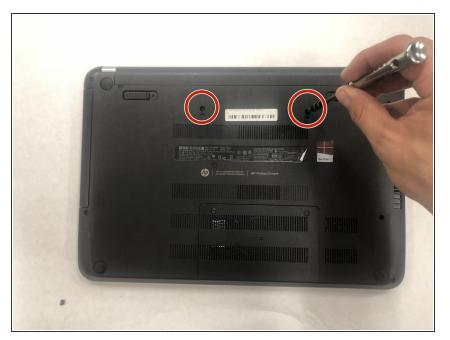
Remove these two, 4 mm long number 1 Phillips screws from the device.
