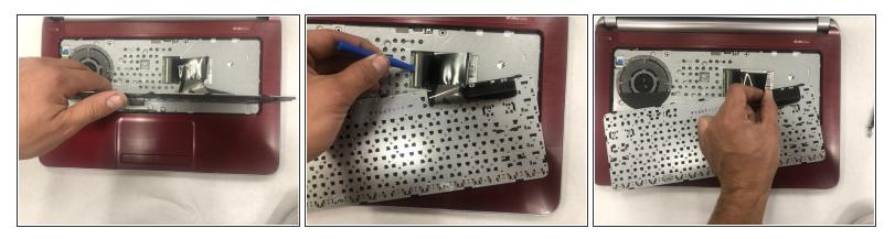
• Lift the plastic retaining tab with a small plastic opening tool. The tab will rotate to the side but not remove from the laptop. After this gently pull the wire ribbon to remove it. The old keyboard is now completely removed.
