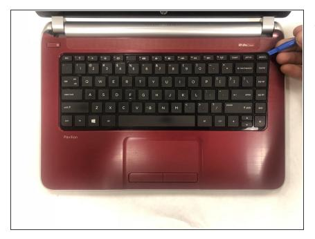
Gently pull the keyboard up with a small plastic opening tool, beginning toward the front right corner. Just pull the keyboard up enough to fit your fingers under.
