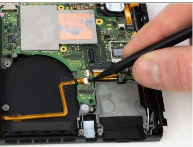
Use a spudger to flip up the small black locking flap on the power/volume ribbon cable <u>ZIF</u> connector.
