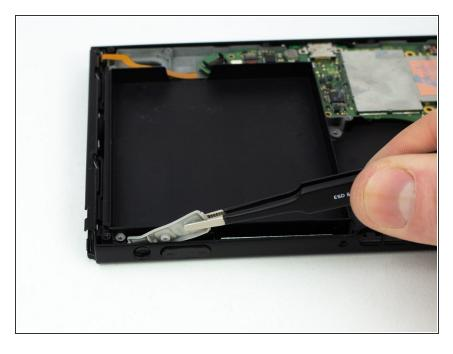
Pull the rubber conductive pad out with a pair of blunt nose tweezers.
