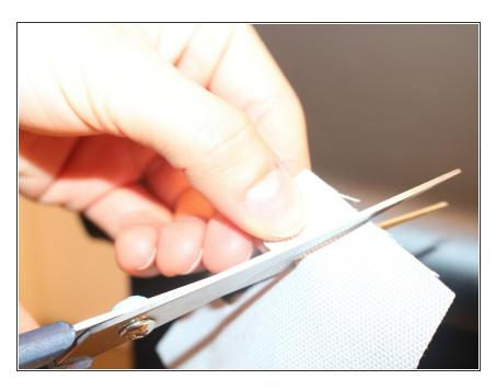
Cut the backing fabric large enough to cover the tear, approximately half an inch larger around the tear.
