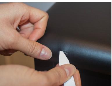
Use the spatula tool to insert the backing fabric underneath the tear.
