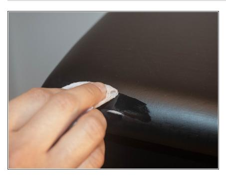
Clean the damaged area with rubbing alcohol, using a rag, paper towel, or Q-tip.
