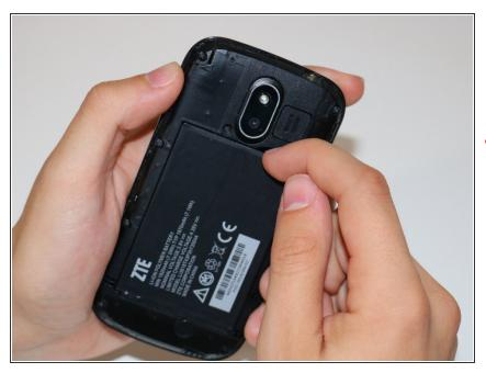
In the top-right area of the battery, use your fingernail to lift the battery out of the phone.
