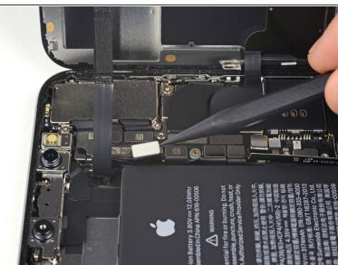
Use the point of a spudger or a fingernail to disconnect the front panel sensor assembly connector.
