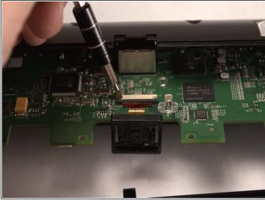
• Use a plastic spudger to push the black sliding cable connector away from the white bracket.
