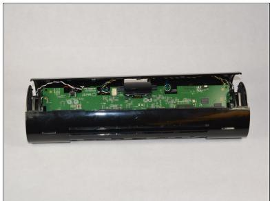
Remove the 1.2 cm hex T9 screws and gently open up the device.
