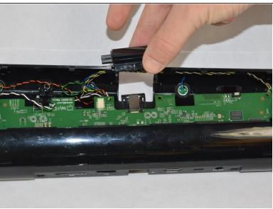
Detach the camera cover from the motherboard. Be very careful to not damage any of the components on the motherboard.
