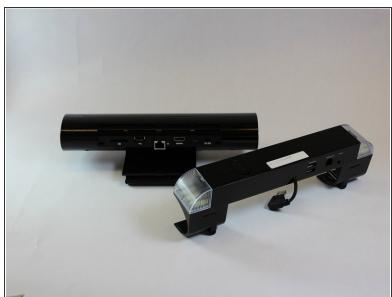
Remove the top bar by removing the 5cm hex T10 screws on the back of the device as shown.
