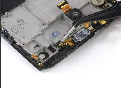
Use a pair of tweezers to gently peel off the cable of the secondary screen at the top of your phone.
