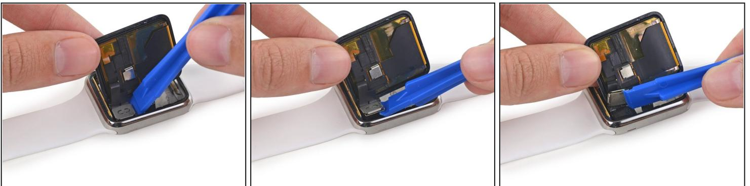
ⓘ The display and digitizer cable connectors are secured beneath a small metal bracket that is adhered to the speaker.
