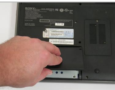
To expose the hard drive, remove the cover by sliding it toward you and pulling up on the panel.
