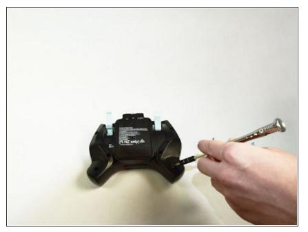
Remove the six screws located on the back of the controller using a JIS #1 screwdriver.
