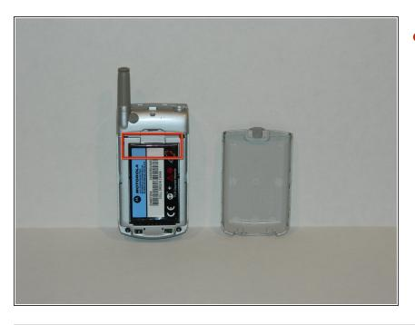
Inserting your finger in the recess at the top edge of the battery, pull the battery away from the housing to remove it.
