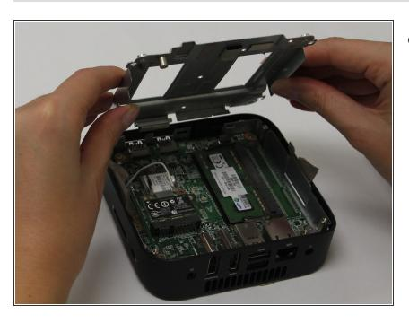
Insert your spudger into the gap between the bottom shield and the ports and gently pry to lift and remove the shield.
