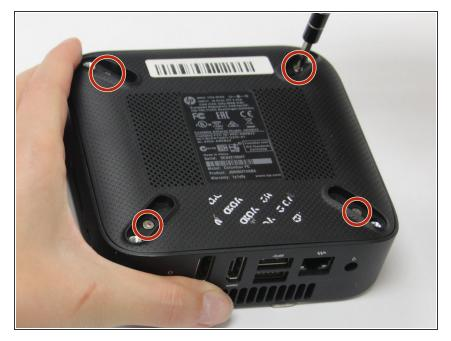
Using your Phillips head screwdriver, remove the four Phillips M2.5×4.0 screws that secure the bottom cover to the computer. In this step the usage of the magnetic mat will be helpful to keep up with the screws.
