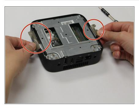
Lift the two pieces of mylar tape from the bracket.
