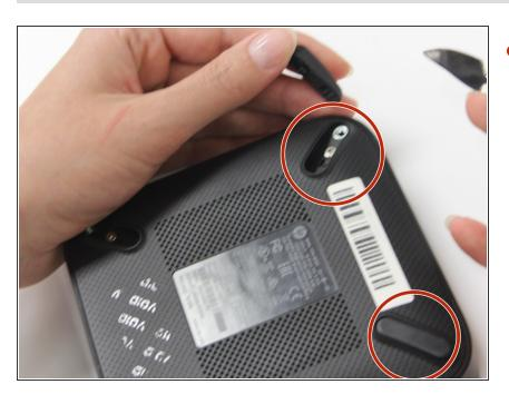
Using your metal spudger, lift and remove the 4 rubber "feet" from each corner.
