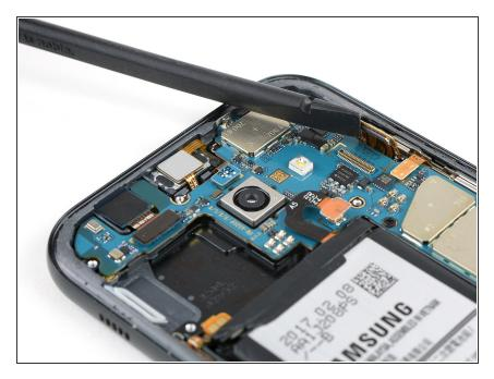
Use the flat end of a spudger and disconnect the display flex cable.
