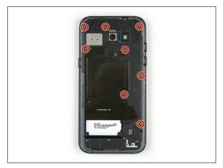
Remove the eight Phillips #00 screws that hold the motherboard cover in its place.
