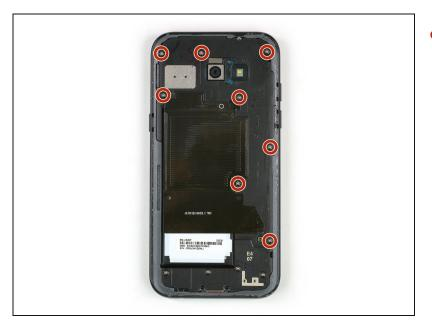
Remove the eight Phillips #00 screws that hold the motherboard cover in its place.
