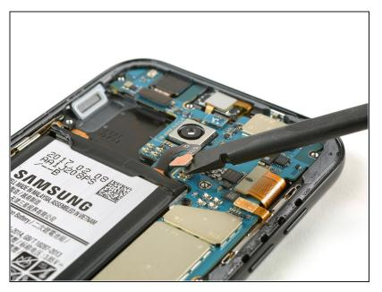
Use the flat end of a spudger to disconnect the battery flex cable.
