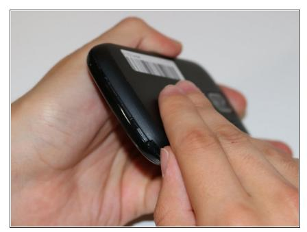
In the bottom right corner of the device, use your fingernail to remove the back cover of the phone by lifting up and holding the device with your other hand.
