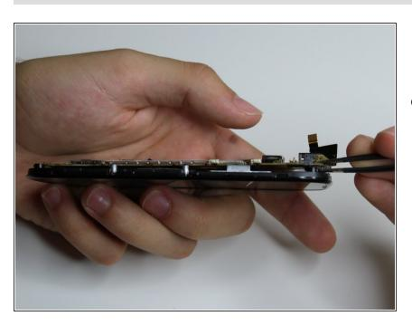
Use your tweezers to disconnect the final ribbon connector underneath the motherboard at the top of the phone. The motherboard can now be separated from the LCD Screen.
