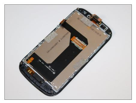
The front screen is separated from the motherboard, so you may replace the front LCD touch screen now.
