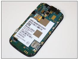
Notice the crease in the shiny black plastic. Insert the flat end of your spudger here, about 3mm above the volume buttons, and work your spudger around the circumference of the phone until the front and back are separated.
