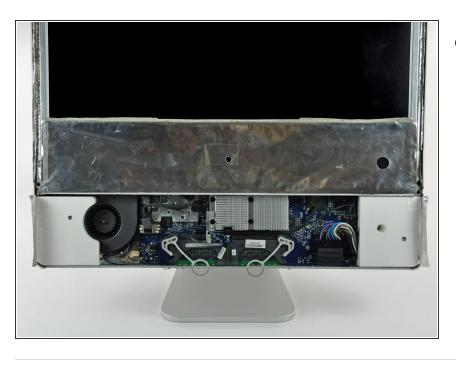
Tape the lower EMI shield up against the face of the display to keep it out of the way while you work.
