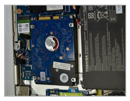
Delicately pull on the hard drive and the case it's in to unplug it from the motherboard.
