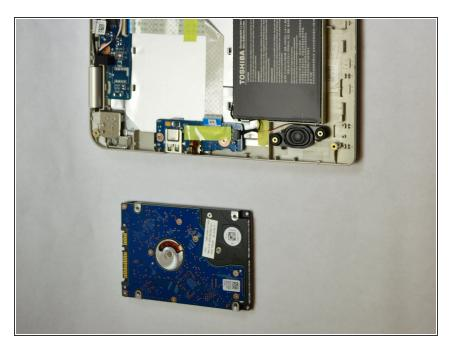
Peal the rubber casing around the hard drive off to completely remove the drive.
