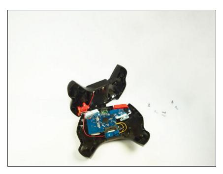
• Pop the front of the controller casing from the back and carefully lay the controller out with circuits exposed.
