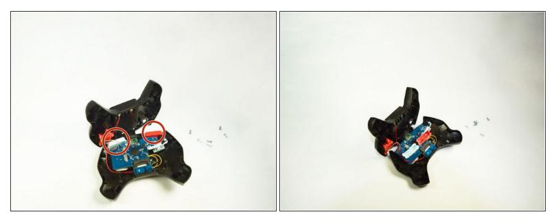
Locate controller buttons at the top of the controller. They are blue and red. Check for debris that may be jamming buttons or broken buttons.
