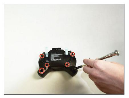
Remove the six screws located on the back of the controller using a #J1 JIS head screwdriver.
