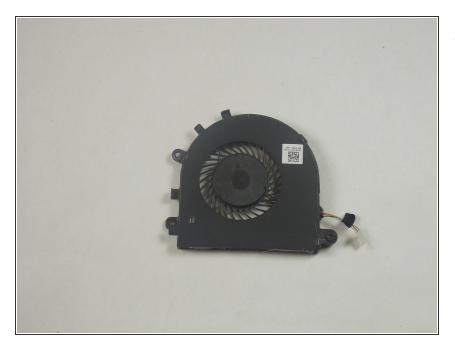
• Lift the fan out of the chassis.
