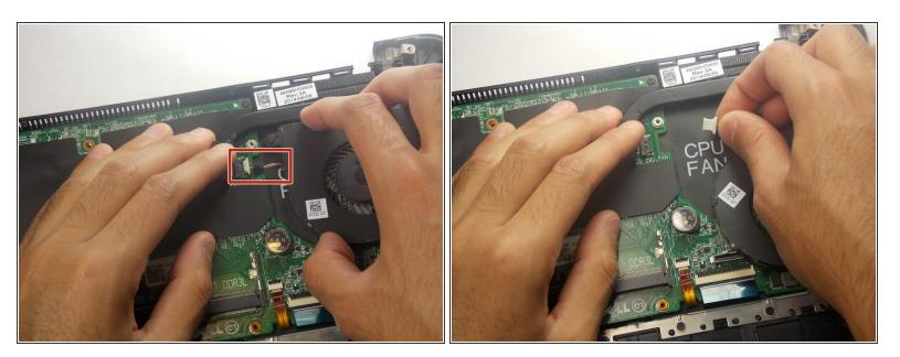
Disconnect the wire that connects the fan to the motherboard. This can be found under the flap directly to the left of the fan.
