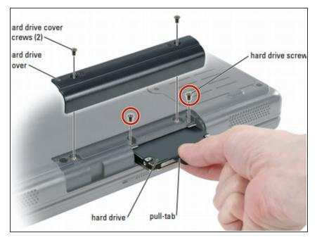
Removing the two screws from the hard-drive.
