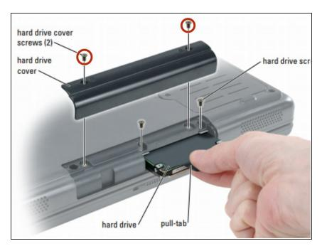
Turn the computer over and remove the hard drive cover screws, the cover, and the hard drive screws.
