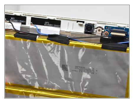
Remove the pieces of black tape that hold the speaker wires to the battery.
