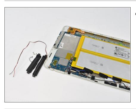
Separate the speakers from the device.
