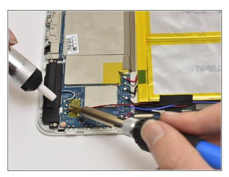
Desolder the speaker wires from the motherboard.
