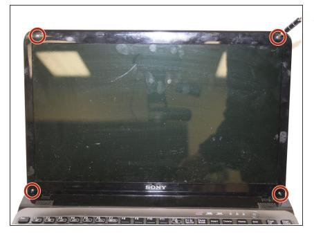
Use a #0 Phillips screwdriver to remove the four 4.0 mm screen bezel screws in each corner.
