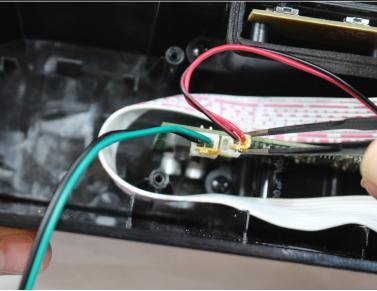
Pull wires out of ports using blunt nose tweezers.
