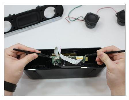
Pull motherboard out of slot using the angled tweezers and blunt nose tweezers on each side.
