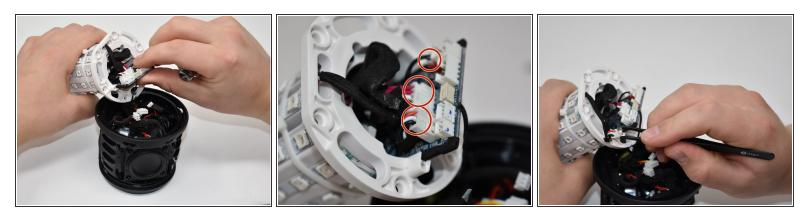
Pull out the motherboard slightly from the LED light display as shown. Using tweezers, unplug the three connections attached to the motherboard.
