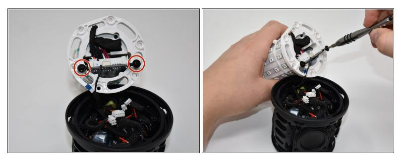
Using a Phillips #0 screwdriver, remove the two black 8mm screws on the bottom of the LED light display.
