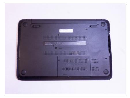
After testing the battery and discovering that it needs to be replaced, you will begin by placing the computer upside-down on a flat surface.
