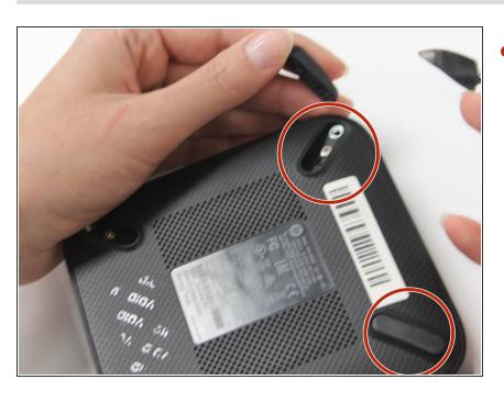
Using your metal spudger, lift and remove the 4 rubber "feet" from each corner.
