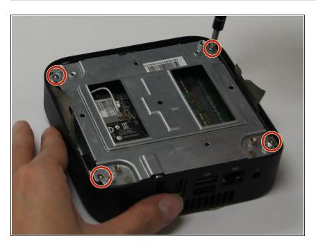
Using your Phillips #1 screwdriver, remove the four Phillips M2.5×4.0 screws that hold the shield in place.
