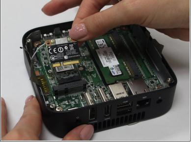
Remove the WLAN module by pulling it away from the slot at an angle.
