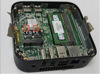
• Disconnect the white and black antenna cables from the module.
