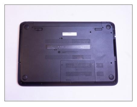
After testing the battery and discovering that it needs to be replaced, you will begin by placing the computer upside-down on a flat surface.
