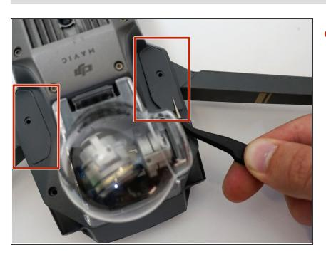
Remove the two small panel pieces near the gimbal case with the tweezers.
