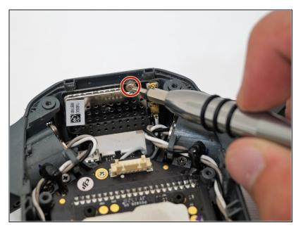
Remove the lone 4mm Phillips #00 screw holding the WiFi board in place by turning the screwdriver counterclockwise.
