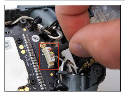
Remove the white connector at the back of the flight controller board by gently pulling at the base.
