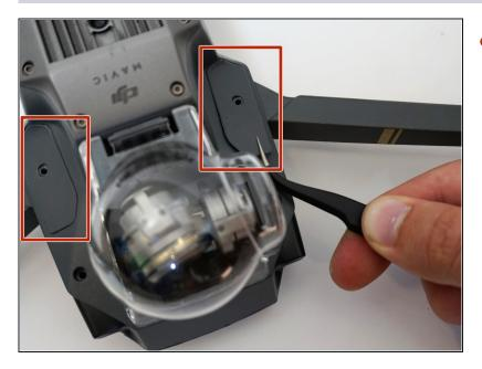
Remove the two small panel pieces near the gimbal case with the tweezers.
