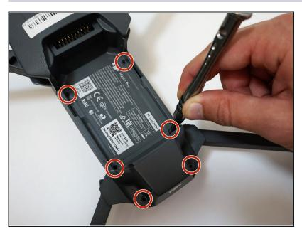
Remove the six 5mm 1.5 Hex screws by turning the screwdriver counterclockwise.
