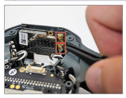
Remove the two gold coaxial connectors by pulling gently at the base with tweezers.
