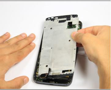
Remove the metal cover by prying underneath it with the opening tool.
