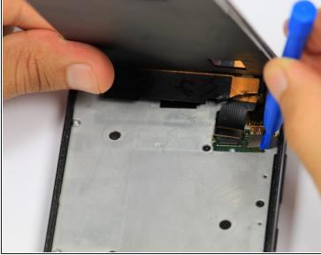
Disengage the two cable connectors by gently prying beneath the edge of the connector with the opening tool.
