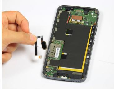
• Remove the fingerprint connector by gently prying underneath the connector with the opening tool.
