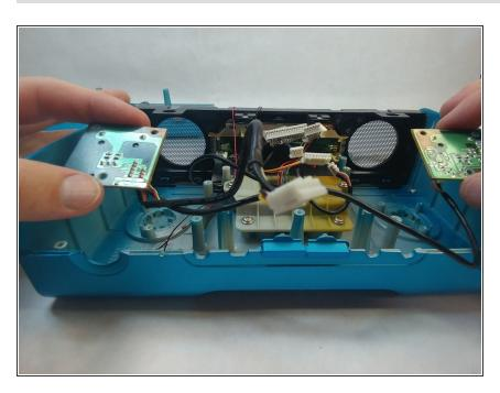
You have successfully removed the scroll wheel circuit boards.
