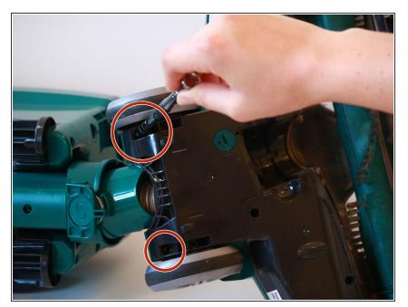
Remove the two 15.9 mm screws from behind the wheels with a T20 bit screwdriver.
