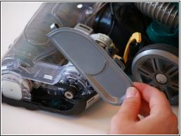
Remove the grey side panel on the motor side of the vaccum with a spudger. Pry under each tab to release the side panel.
