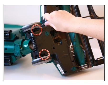
Remove the two 14.3 mm screws under the wheels with a T20 screwdriver bit.
