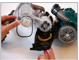
Remove the visible side of the belt from the gear with a spudger.
