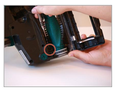
Remove the single 13.4 mm screw from behind the belted end of the roller brush with a T20 screwdriver bit.
