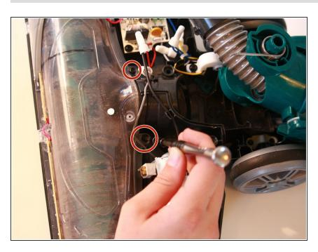
Remove the two 13.4 mm screws with a T20 bit screwdriver.
