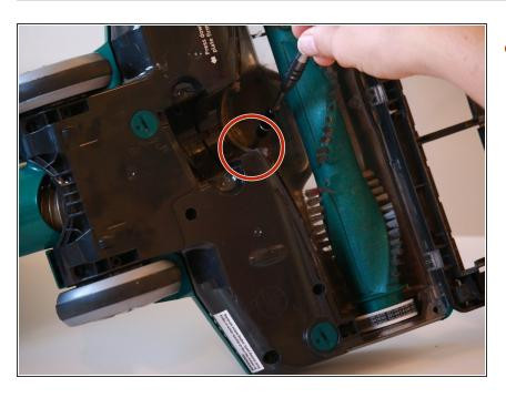
Remove the single 13.4 mm small screw behind the roller brush with a PH0 screwdriver bit.
