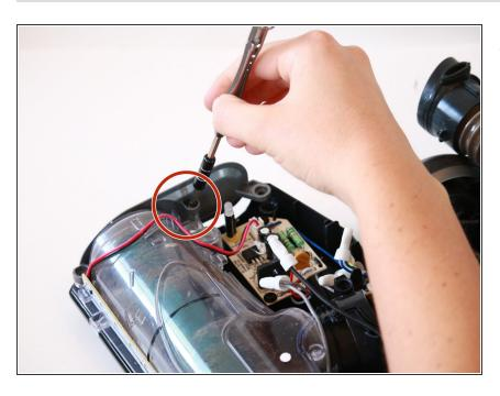
Remove the grey panel from the opposite side, by uncrewing the single 13.4 mm screw with a PH1 screwdriver. This will release the container for the roller brush and belt motor.
