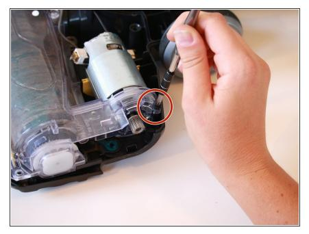
Remove the single 13.4 mm screw located next to where the belt was detached, securing the motor in place, with a PH1 screwdriver.
