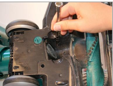
Remove the three 14.3 mm screws with a T20 screwdriver.
