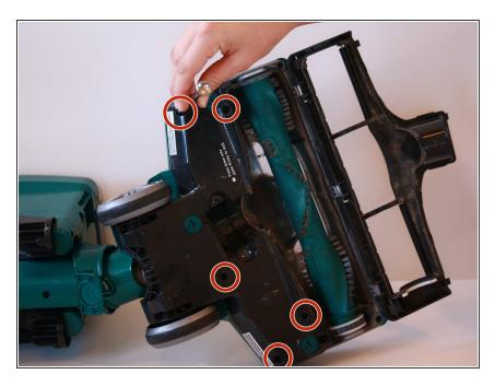
Using a T20 screwdriver, remove the five 15.9 mm screws on the outside cover.
