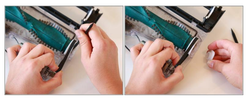
Using the spudger, push the white end cap out of the clear plastic by placing the spudger on the roller brush side and pushing the cap outward.
