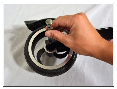
• Flip over the scooter and use the hex bit 4.0 to remove the other 0.2 mm screw.
