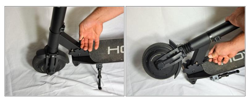
• Fold the scooter by releasing the latch and pushing the handlebars to the rear of the device.
