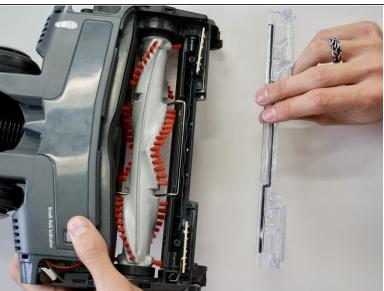
Use the metal spudger to pry off the clear, plastic cover on the LEDs.
