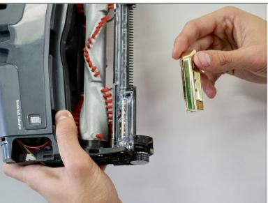
Use the nylon spudger to pry the gold, plastic cover off of the headlights.
