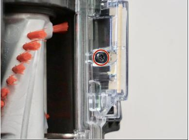
Turn the T10 Security Torx screwdriver counterclockwise to remove the 15mm screw.
