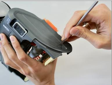
Remove the plastic screw covering using a metal spudger by pushing the sharp side into the crevice and prying the cover out.
