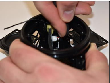
Disconnect the two connections from the inside side of the base of the JBL Pulse 3 by pushing on the wire with your index finger in the opposite direction of the connection.
