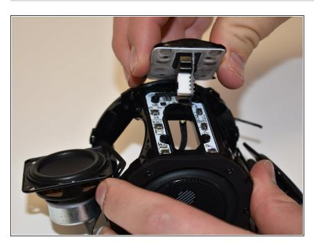
Pull off the inside button cover with the attached charging port. The charging port should now be removed.
