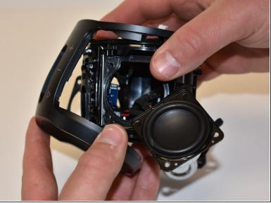
Grab the outside of the JBL Pulse 3 at the bottom and pull outward until the outside button cover comes off.
