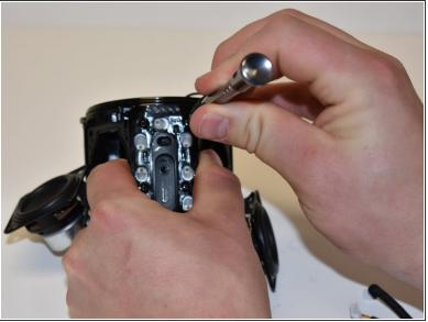
Using a Phillips #1 screwdriver, remove the four 10mm screws by the push buttons on the side of the base of the JBL Pulse 3.
