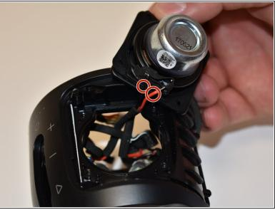
Pull out the speaker and cut the black and red wire with wire cutters. The speaker should now be removed from the JBL Pulse 3.
