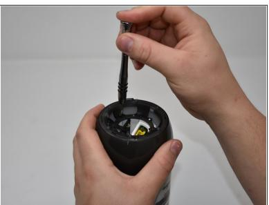
• Remove the five 7mm screws on the inside of the JBL Pulse 3 with a Phillips #1 screwdriver.
