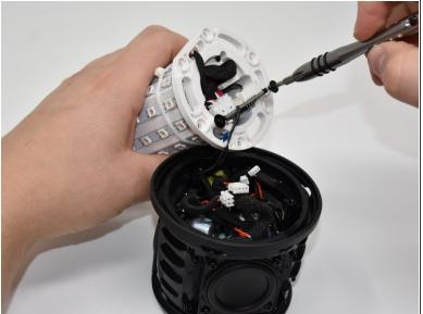
Using a Phillips #0 screwdriver, remove the two black 8mm screws on the bottom of the LED light display.
