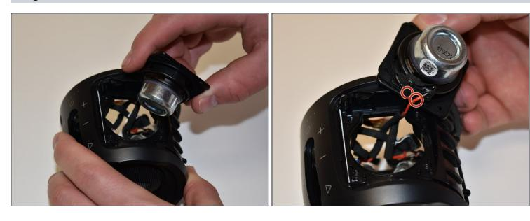
• Pull out the speaker and cut the black and red wire with wire cutters. The speaker should now be removed from the JBL Pulse 3.
