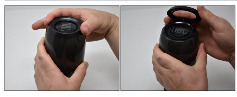
• Turn the JBL Pulse 3 right-side up and unscrew the top ring of the device. A small amount of force and/or a cotton cloth may be necessary to remove this piece.
