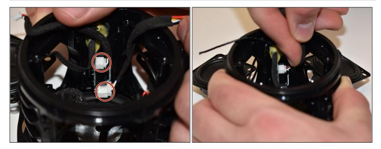
• Disconnect the two connections from the inside side of the base of the JBL Pulse 3 by pushing on the wire with your index finger in the opposite direction of the connection.
