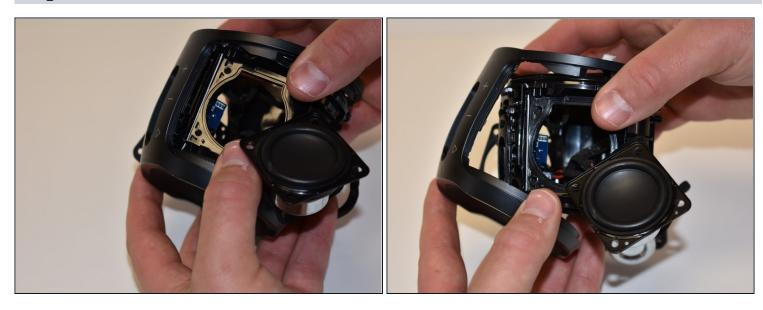
• Grab the outside of the JBL Pulse 3 at the bottom and pull outward until the outside button cover comes off.
