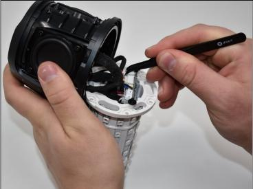
Use tweezers to pull the five connections off of the LED light display.
