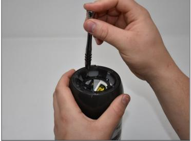
• Remove the five 7mm screws on the inside of the JBL Pulse 3 with a Phillips #1 screwdriver.
