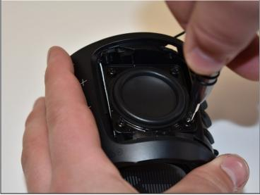
• Using a Phillips #2 screwdriver, remove the four 10mm screws on the corner of the speaker on the side of the base of the JBL Pulse 3.
