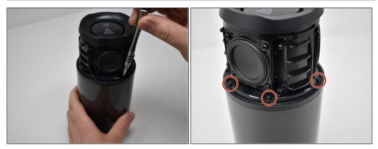
• Use a Phillips #00 screwdriver to remove the six black 6mm screws on the inside of the top of the bottom section.
