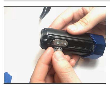
Remove the power button from the device.
