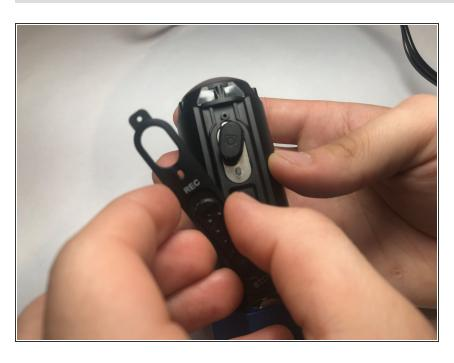
Lift off the plastic part holding the power button in place.
