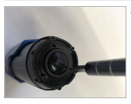
Remove the 3 screws that secure the camera to the body using a #00 Phillips screwdriver.
