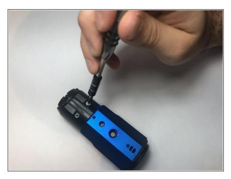
Remove 2 screws on the bottom of the camera body using a #00 Phillips screwdriver.
