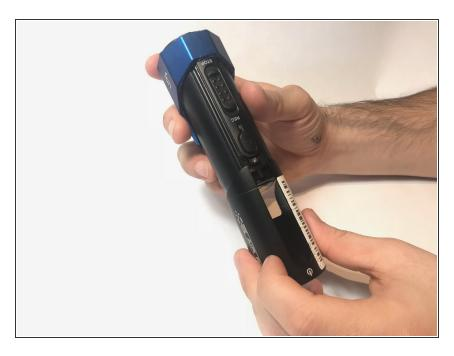
Remove the metal camera body cover by sliding it toward the lens end of the camera.
