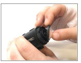
Remove the 6 screws securing the lens cover bezel using a #00 Phillips screwdriver. This will allow you to remove the bezel and lens cover.
