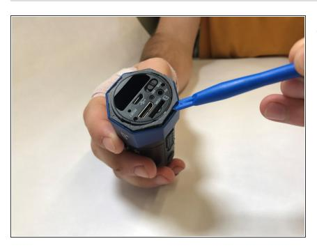
Use a plastic pry tool to remove the plastic ring covering the rear screws.
