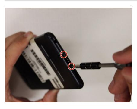
Remove the two 2 mm screws using a Torx T2 screwdriver.
