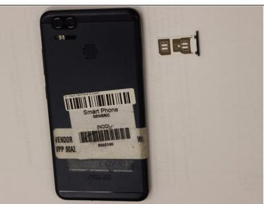
Using a pair of tweezers, pull put the SIM card tray and set it to the side.
