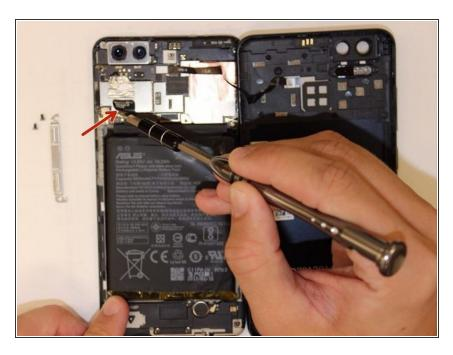
Disconnect the battery connections.
