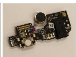
• Using the pry tool, pry up the circular piece and remove the board.
