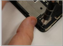
Remove all screws 3mm, using the Phillips #00 screwdriver, at the bottom of the device.
