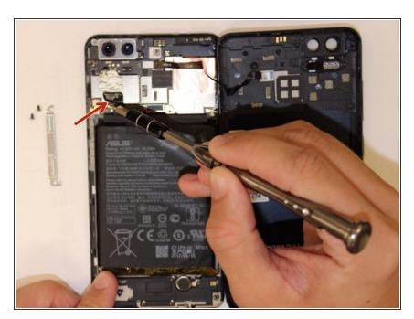
Disconnect the battery connections.
