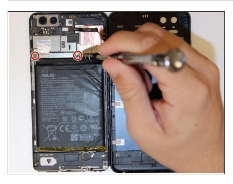
Remove the two 3 mm screws, using the Phillips #00 screwdriver, on the silver band at the top of the battery and remove the band.
