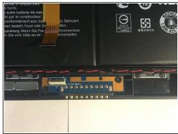
Flip the latch and carefully pull the ribbon free.
