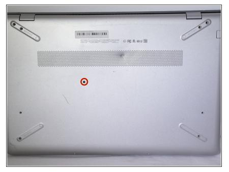
Use a PH000 screwdriver to remove the 4mm screw that secures the optical drive.
