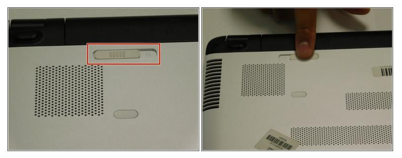
Unlock the battery by moving the tab to the unlock position.
