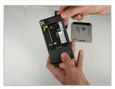
The battery has been successfully removed.
