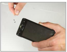
Use a T5 Torx screwdriver to remove the screws in each corner of the phone.
