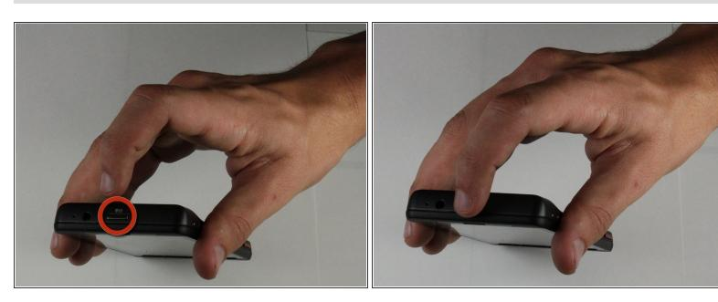
Locate the power button at the top of the phone. Depress power button for 2 seconds until a menu appears.
