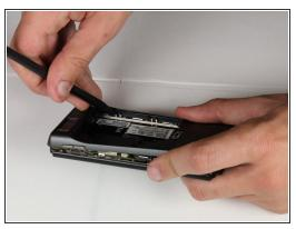
Locate the two clips on the inside of the case and use the spudger tool to detach them from the case. To detach each clip, use the sharp end to press the small, black plastic in the center of the clip.
