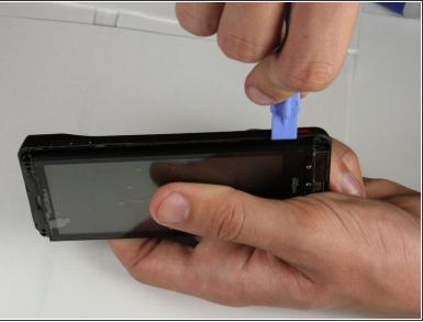
Locate the seam along the right edge of the phone. Use the prying tool to disconnect the two clips along the edge.
