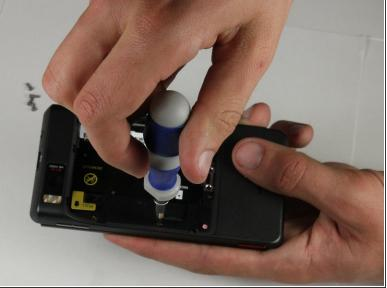
Flip the phone over and locate the screw on the middle of the left side. Unscrew it using the T5
