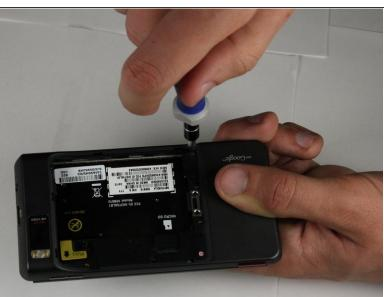
Identify the screw located in the bottom right corner of the battery case. Remove the screw with a T5 (or in some cases T6) torx screwdriver and set it aside.
