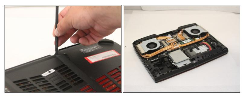
Using the black nylon spudger, carefully remove the rear cover from the laptop.
