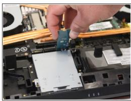
Using the Phillips #0 screwdriver, remove each screw from the SSD card units, then unplug and remove them. The screws are 0.25 inches long.
