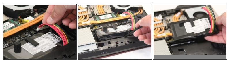
Carefully unplug the battery and remove it from the laptop. This will be held down with adhesive, but can be safely removed once unplugged.
