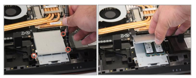
Using the Phillips #0 screwdriver, remove each screw from the heatsink and remove it.
