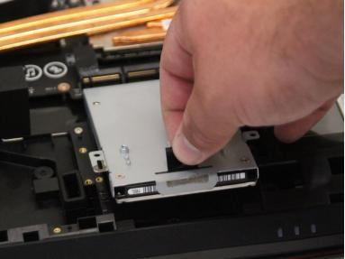
Remove all screws from the back of the hard drive using the Phillips #0 screwdriver, then lift up and unplug the unit. Screws are 0.15625 inches long.
