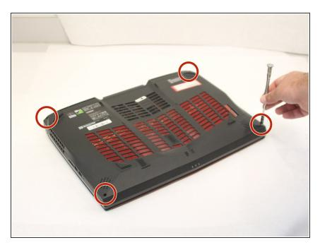
Remove the four rear screws using the Phillips #0 screwdriver from the laptop as shown. The screws are 0.5 inches long.
