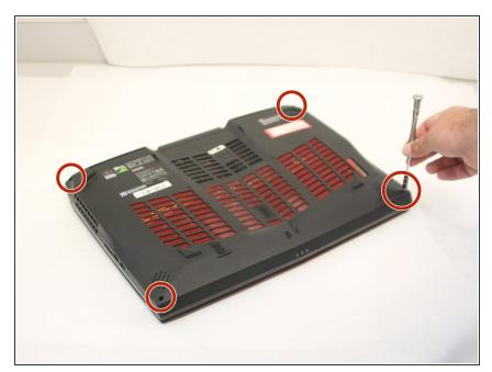
Remove the four screws from the back cover using the Phillips #0 screwdriver. Screws are 0.5 inches long.
