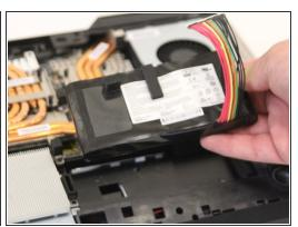
Unplug the battery, then using the black nylon spudger, carefully remove it from the laptop. It is held down by an adhesive, but can be safely removed without damaging the device.
