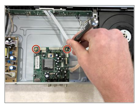
Remove the two 7.94 mm #1 Phillips head screws from the motherboard.
