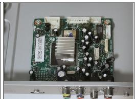
Unplug the one ribbon wire and the five bundled cable connectors that are plugged into the motherboard.
