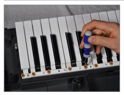
Completely unscrew and remove the screws holding the broken string of keys in place.
