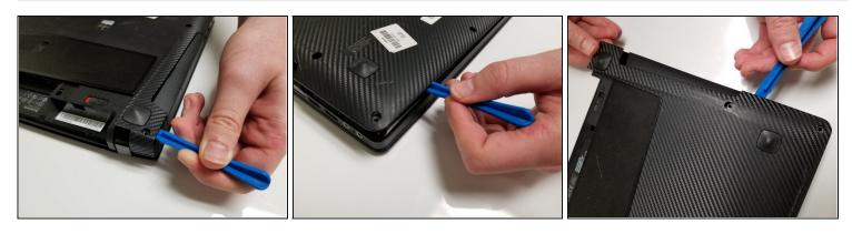
Use the plastic opening tool to remove the back panel from the device.
