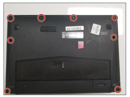
Remove the eight 9mm screws with a Phillips #0 screwdriver.
