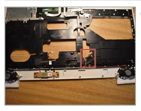
Follow the red and white wires until they join into a plug and disconnect for easy removal of the speakers.
